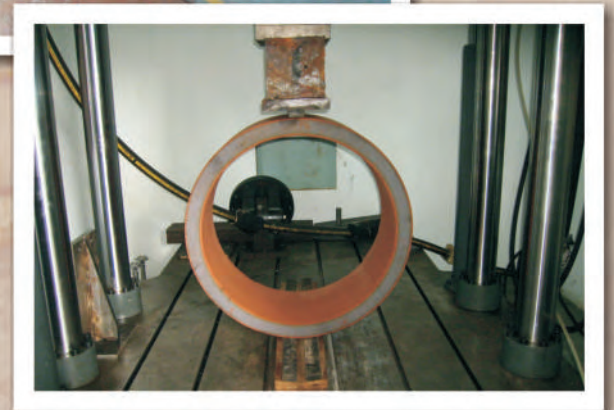
Pipe being type tested in accordance with EN295-7 Clause 4.8 Strength
